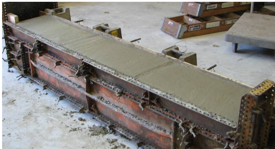
Figure 19. Finished concrete surface of Type 1 Connection.
