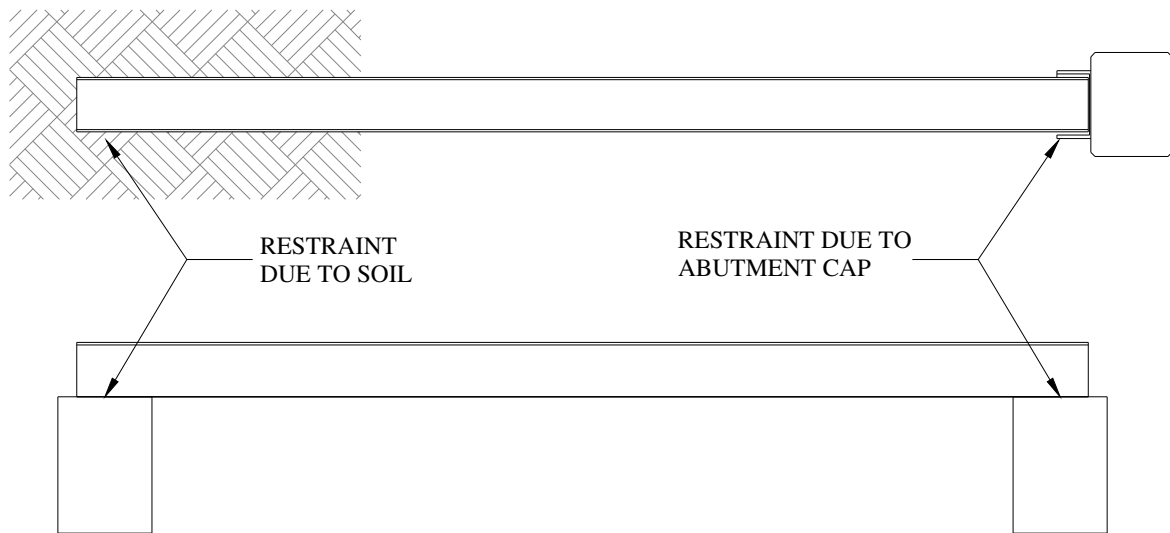
Figure 38. Correlation of field conditions to the laboratory set-up.
