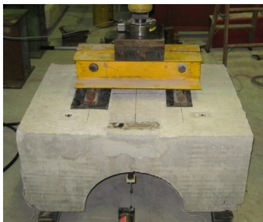
b) Photograph of ultimate load test
