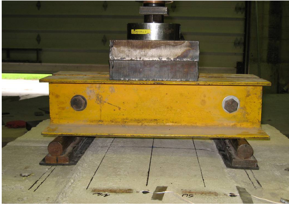
Figure 35. Ultimate load test set-up.
